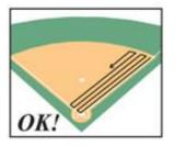
IMPORTANT: It is critical to alternate dragging patterns to not move material consistently in one direction. This will help slow lip development and crown degradation.
